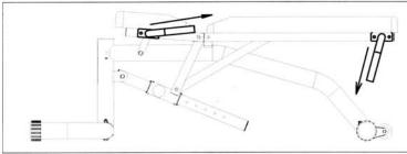
Note 1: See diagram at left. Be sure that seat pad handles point upward on each side, and back pad handles point downward and forward when bench is in flat position.
